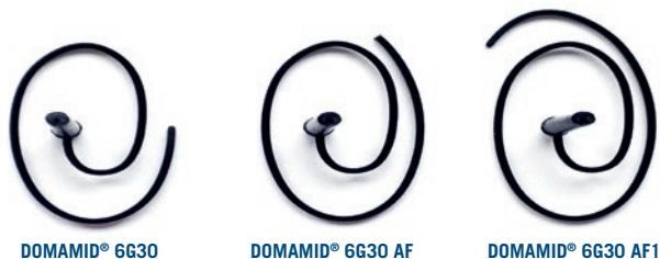
The clear improvement in the flow properties of DOMAMID® AF and AF1 products can be seen in the length of the flow spiral.
